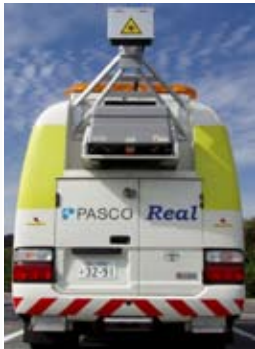
The PASCO REAL system incorporates a stereo camera, POSLV, line scan camera, laser scanner, distance sensor and generator.
