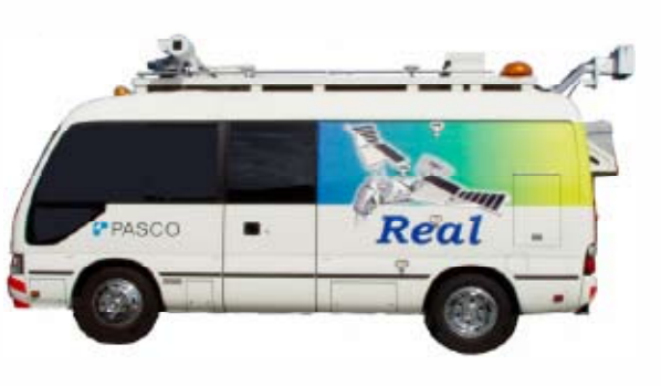
The PASCO REAL system incorporates a stereo camera, POSLV, line scan camera, laser scanner, distance sensor and generator.
