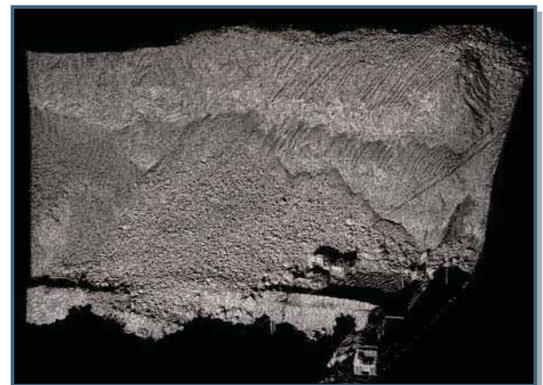
Overspill volume calculation is easily and accurately generated, a task which is virtually impossible without the use of lidar. Right: Unrendered point cloud of a typical overspill.
