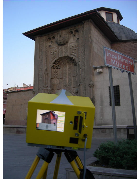
Figure 6. ILRIS-3D and measurement of Ince Minare Medresesi
